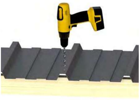
First pre-drill the roofing sheet using TABLE A. Next pre-drill the substructure using TABLE B.
